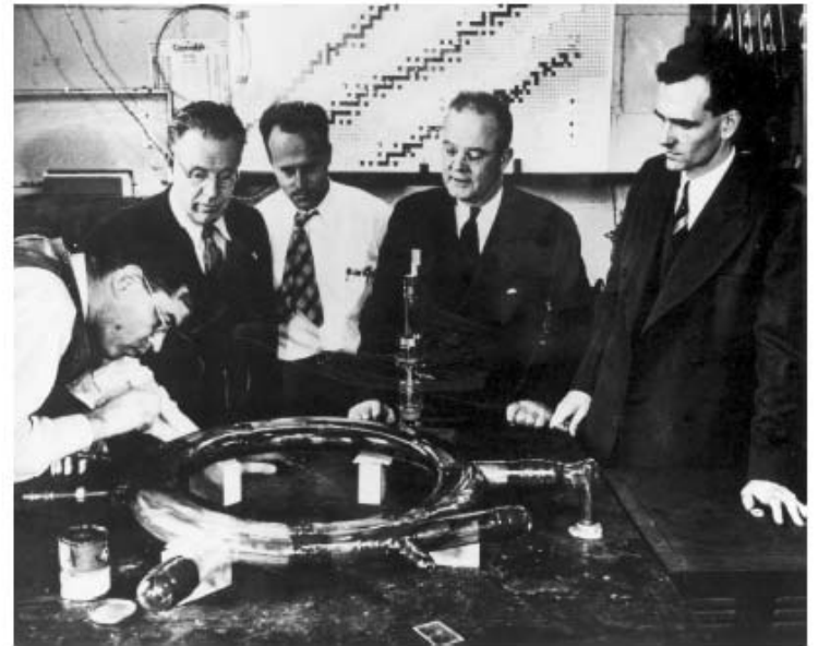
Figure 5 The General Electric team (from left to right, Langmuir, Elder, Gurewitsch, Charlton and Pollock) looking at the vacuum chamber of the 70 MeV synchrotron – the world's second synchrotron.
